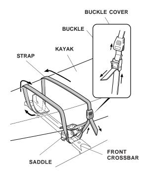
8. Route the strap under the rear crossbar, and around the kayak as shown. Slide the buckle cover away from the buckle, route the strap through the buckle, and tighten the strap. Slide the buckle cover back over the buckle.
