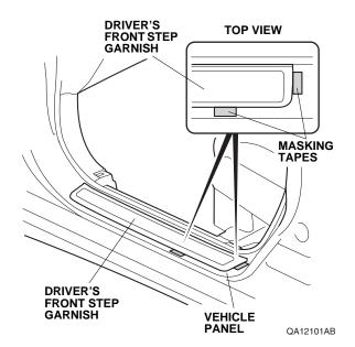
16. Pull away the door opening seal, and remove and discard the driver's front step garnish.
