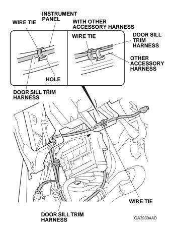
53. Route the door sill trim harness, and secure it to the vehicle frame with one wire tie.
