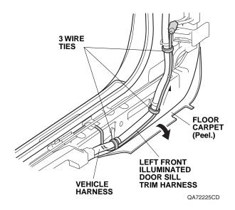
48. Route the left front illuminated door sill trim harness, and secure it to the vehicle harness with three wire ties.
