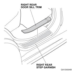
35. While applying light pressure against the right rear door sill trim, carefully remove the adhesive backings.
