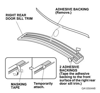
33. Using one alcohol swab, thoroughly clean the right rear step garnish where the right rear door sill trim will attach.
