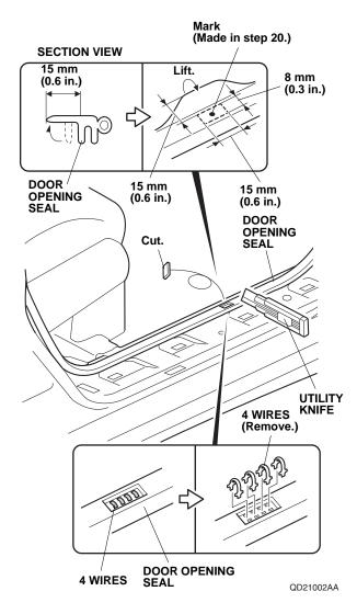
23. Remove the four wires from the part of the door opening seal.
