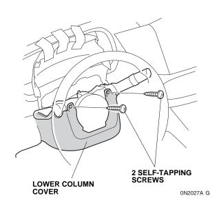
10. Remove the lower column cover (one self-tapping screw).
