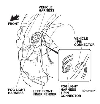
27. Secure the fog light harness to the vehicle harness with two wire ties.
