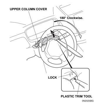
Secure the upper column cover to the meter panel 8. with the tape.
