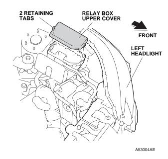
59. Using isopropyl alcohol on a shop towel, thoroughly clean the area where the fuse label will attach. Attach the fuse label to the relay box upper cover.
