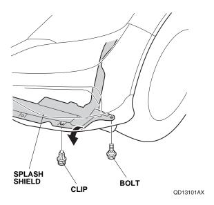
2. Insert your hand inside of the splash shield released in step 1. Unplug the connector from the fog light.
