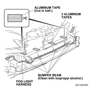
34. Using scissors, cut one aluminum tape in half. Secure the fog light harness to the bumper beam with two pieces of halved aluminum tape. 35. Route the fog light harness, and secure one clip on the fog light harness to the vehicle panel.
