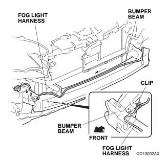
33. Using isopropyl alcohol on a shop towel, thoroughly clean the areas where the aluminum tapes will attach. Secure the fog light harness to the bumper beam with three aluminum tapes.
