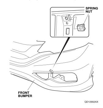
23. Install the left fog light to the front bumper with two hooks and one self-tapping screw. Hook the two hooks in the order shown.
