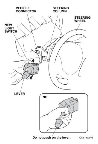
55. Plug the vehicle connector to the new light switch. Make sure the vehicle harness is not being stretched. 56. If a 20A fuse is already installed in the fuse box, go to step 58, otherwise, plug the 20A fuse into the fuse box.
