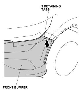
• On each side, release the four retaining tabs.
