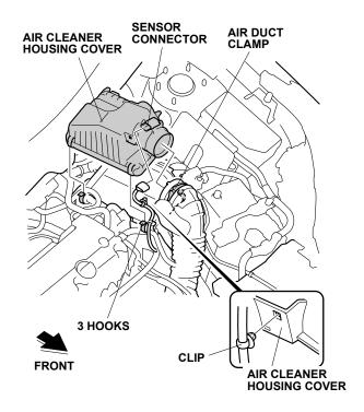
26. Remove the air cleaner housing (one bolt and two pins).
