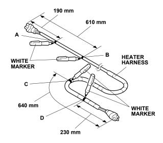
39. Plug the heater harness connector to the engine block heater. Make sure that the heater harness connector is properly installed.
