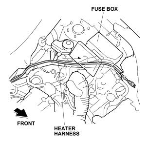
43. Route the heater harness forward along the vehicle harness.
