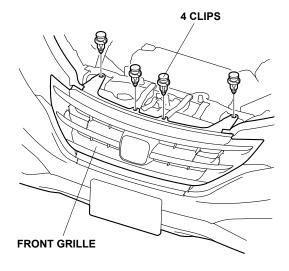
11. Using a flat-tip screwdriver, release the four clips from the bottom of the front grille.
