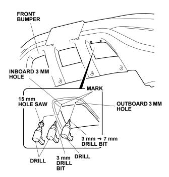
50. Using a 7 mm drill bit, enlarge the outboard 3 mm hole to 7 mm. Using a 15 mm hole saw, enlarge the inboard 3 mm hole to 15 mm.
