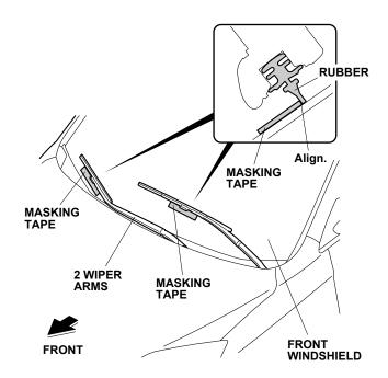
15. Remove the two windshield wiper arms (two caps and two nuts). Wiper arm nut torque is 29.4 N·m (21.6 lbf·ft).
