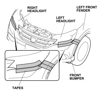
9. Attach masking tape to the front grille and front bumper in the area shown.
