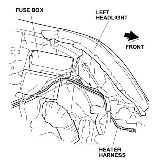
44. Route the heater harness through the front bulkhead as shown.
