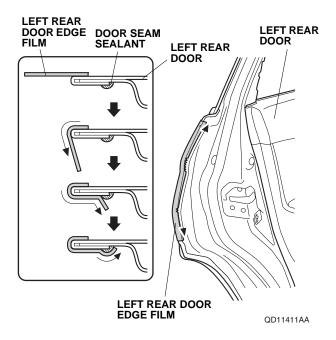
18. Using a shop towel, wipe the excess 3M protective tape application solution from the left rear door edge film. Allow the left rear door edge film to dry thoroughly.
