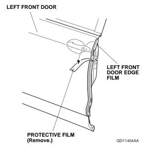
10. Starting from the center and working outward, use your finger to fold the left front door edge film inside the left front door. Move your finger in one direction only. Do not damage the door seam sealant.
