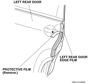
17. Starting from the center and working outward, use your finger to fold the left rear door edge film inside the left rear door. Move your finger in one direction only. Do not damage the door seam sealant.
