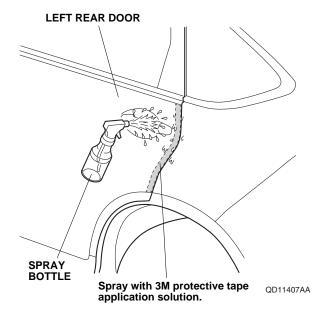
13. Open the left rear door. Peel back about 50 mm (2.0 in.) of adhesive backing from the left rear door edge film. Align the V-notch on the left rear door edge film with the character line on the left rear door.
