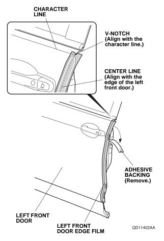
7. Align the center line on the left front door edge film to the edge of the left front door. While applying light pressure, carefully remove the adhesive backing.
