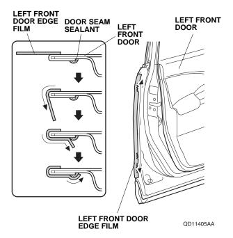
11. Using a shop towel, wipe the excess 3M protective tape application solution from the left front door edge film. Allow the left front door edge film to dry thoroughly.
