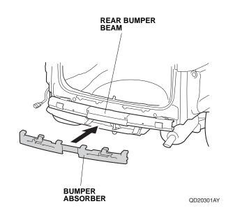
90. With the help of an assistant, bring the rear bumper to the vehicle, and plug the backup sensor harness 8-pin connector into the subharness 8-pin connector. Reinstall the rear bumper.
