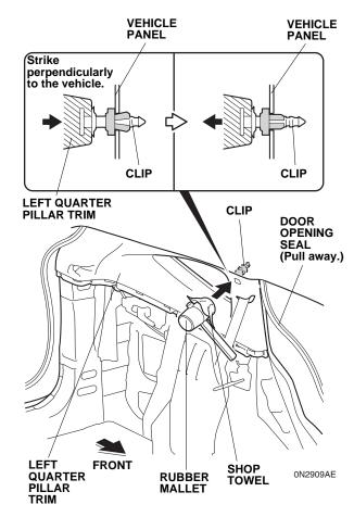
19. Using a rubber mallet wrapped with a shop towel, lightly tap the area marked "SIDE CURTAIN AIRBAG" on the left quarter pillar trim to push in the clip. Make sure to strike area perpendicularly to the vehicle. 20. Remove the left quarter pillar trim.
