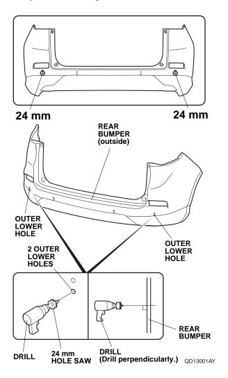
75. While wearing eye protection and drilling from painted side of the rear bumper, enlarge the two lower 3 mm inner holes to 26 mm using a 26 mm hole saw.
