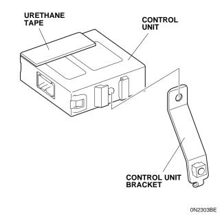
35. Using isopropyl alcohol on a shop towel, thoroughly clean the control unit where the urethane tape will attach. Attach the remaining piece of urethane tape (cut in step 33) to the control unit in the area shown.
