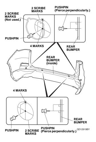
73. While wearing eye protection, drill the eight pierced marks with a 3 mm drill bit from the painted side of the rear bumper.
