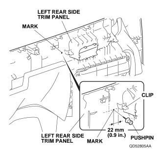
63. While wearing eye protection, drill the pierced mark on the left rear side trim panel with a 3 mm drill bit. Enlarge a 3 mm hole to 26 mm using a 26 mm hole saw. Remove any burrs.
