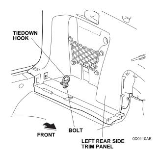
16. Pull away the weatherstrip from around the left rear side trim panel at the tailgate, and remove the door opening seal at the left rear door. Starting at the front, release the left rear side trim panel.
