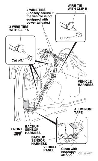
39. Route the backup sensor harness up along the vehicle harness, and secure it to the vehicle harness with three wire ties with clip A, one wire tie with clip B, and two wire ties as shown. If the vehicle is not equipped with the power tailgate, loosely secure the two wire ties. Go to step 42.
