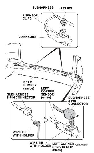
82. Install the wire tie with holder to the subharness 8-pin connector, and secure it to the left corner sensor clip (black) as shown. 83. On the inside of the rear bumper, using isopropyl alcohol on a shop towel to thoroughly clean the rear bumper where the aluminum tapes will attach.
