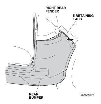
• On each side, release four retaining tabs.
