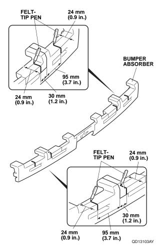
88. Using an utility knife, cut out the bumper absorber along the mark on each side of the bumper absorber.
