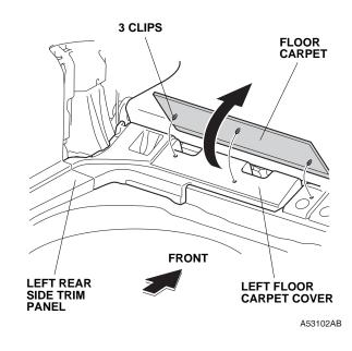
11. Remove the left floor carpet cover (three clips and two retaining tabs).
