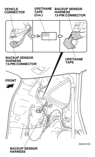
44. Using scissors, cut one urethane tape as shown. Attach the cut piece of urethane tape to the backup sensor harness 13-pin connector. If the vehicle is equipped with the trailer hitch harness, continue with step 45; otherwise, go to step 48.
