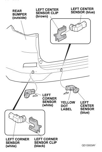
77. Secure the left corner sensor (white) and left center sensor (blue) with left corner sensor clip (black) and left center sensor clip (brown) as shown.
