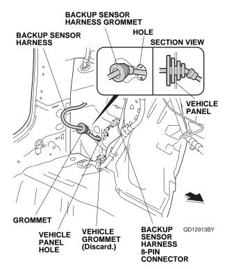
30. Route the backup sensor harness 8-pin connector through the hole, and seat the backup sensor harness grommet into the vehicle panel hole. NOTE: Do not pull on the backup sensor harness when installing the grommet.
