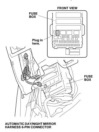
18. Unplug the other accessory 6-pin connector from the fuse box, and plug the automatic day/night mirror harness 6-pin connector into the fuse box.
