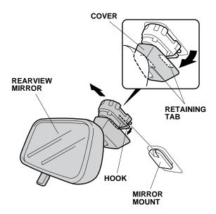
4. While holding down the hook, remove the rearview mirror from the mirror mount as shown.
