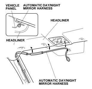
28. Align the green tape on the automatic day/night mirror harness with the edge of the headliner. Be careful not to crease the headliner.
