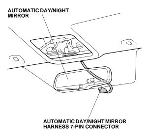
32. Route the automatic day/night mirror harness through the grooves in the harness cover. Secure the harness cover to the mirror stay as shown.
