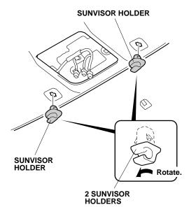
6. Rotate each sunvisor holders 45° counterclockwise to remove the two sunvisor holders.
