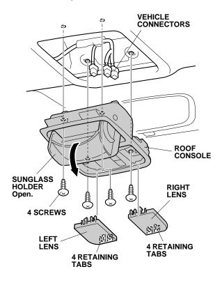
3. Remove the cover (two retaining tabs).
