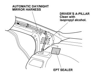
27. Gently pull down the headliner, and tuck the automatic day/night mirror harness under the headliner. Be careful not to crease the headliner.
