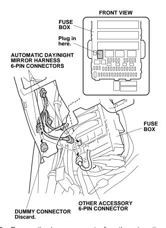
Remove the dummy connector from the automatic day/night mirror harness 6-pin connector, and plug the other accessory 6-pin connector to the automatic day/night mirror harness 6-pin connector. 20. Route the automatic day/night mirror harness as shown.
