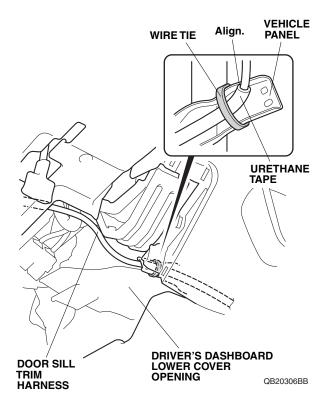
62. Secure the door sill trim harness to the vehicle harness with one wire tie. Move the steering wheel up and down through its full adjustment range and make sure the door sill trim harness is not being stretched.
