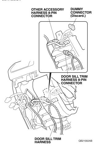
42. Route the door sill trim harness as shown, and secure the door sill trim harness to the vehicle harness with one wire tie.
