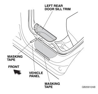
36. While applying light pressure against the left rear door sill trim, carefully remove the adhesive backings.
