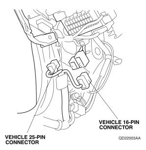
44. Plug the vehicle 25-pin connector into the door sill trim harness 25-pin connector. Plug the door sill trim harness 25-pin connector into the vehicle 25-pin connector.
