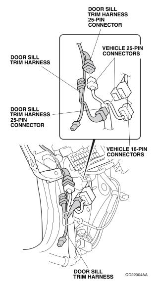
45. Re-plug the vehicle 16-pin connector.
