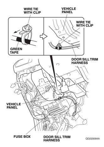
54. Using diagonal cutters, cut the clip portion off of one wire tie.
