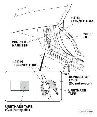
68. Secure the 2-pin connectors to the vehicle harness with one wire tie.
