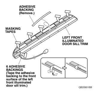
19. Using one alcohol swab, thoroughly clean the vehicle panel where the left front illuminated door sill trim will attach.
