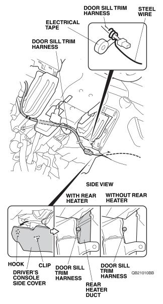
58. Attach a piece of steel wire to the door sill trim harness with electrical tape. Route the door sill trim harness through the center console from the driver's dashboard lower cover opening to the passenger's under cover opening.
