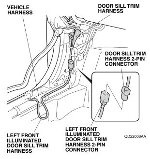
48. Plug the left front illuminated door sill trim harness 2-pin connector into the door sill trim harness 2-pin connector.
