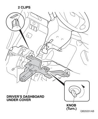
6. Remove the driver's dashboard lower cover and unplug the vehicle connectors.
