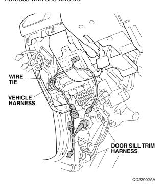
43. Unplug the vehicle 16-pin connector and 25-pin connector.
