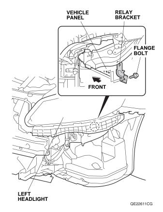
41. Install the case on the relay bracket.
