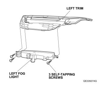
21. Install the left trim on the front bumper with nine retaining tabs and one clip.
