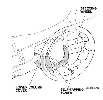
6. Turn the steering wheel 180° clockwise, and remove the other self-tapping screw from the lower column cover.
