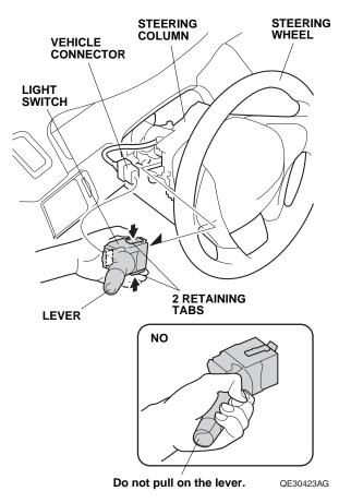
Push down on the two retaining tabs, slide the light switch out, and remove it from the steering column. Do not pull on the lever.  Install the new light switch on the steering column. Make sure both retaining tabs are locked in place. Do not push on the lever.
