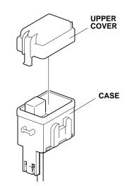
36. Route the fog light harness through the case, and install the relay block in the case.
