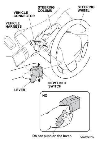
11. Plug the vehicle connector into the new light switch. Make sure the vehicle harness is not being stretched. 12. Attach masking tape to the areas shown.
