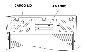
3. While wearing eye protection, drill the four marks from the underside with a 3 mm drill bit, then enlarge the holes with a 10 mm drill bit from the top. Remove all burrs.
