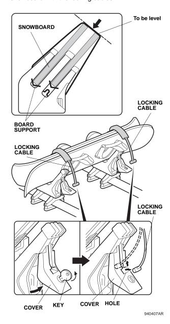
12. Check that the locking cables are inserted securely, then close the covers.
