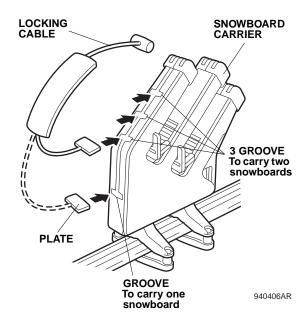
11. Load the snowboard on the carrier, adjust it so that the top edges are level and the boards are as far down in the carrier as possible. Secure the snowboard with the locking cables.
