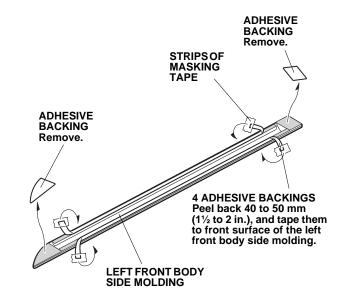
Align the edges of the left front body side molding with the edges of the front template, and install the left front body side molding on the left front door.
