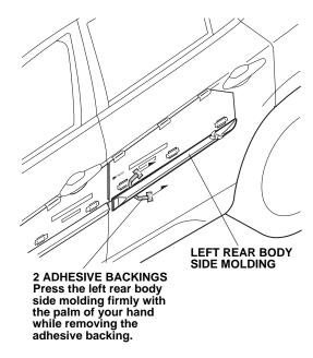
Using the rubber roller, apply firm pressure, especially at the ends, while rolling to set the adhesive.
