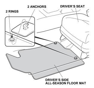
**4WD model:** Place the grommets in the driver's side all-season floor mat over the tabs, and turn the tabs one quarter turn to secure the all-season floor mat.
