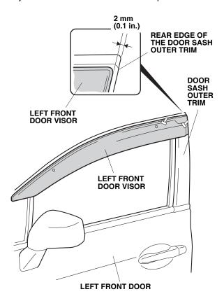
While applying light pressure against the left front door visor, carefully remove the adhesive backings.
