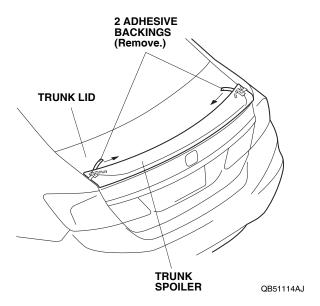
22. Using your hand, firmly press this portion of the trunk spoiler against the trunk lid.
