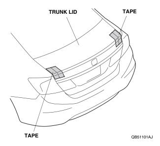
Place the template on the left side of the trunk lid, and align the template with the edge of the trunk lid as shown. Tape the template to the trunk lid with strips of masking tape.
