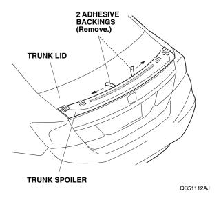
18. Using your hand, firmly press the top center portion of the trunk spoiler against the trunk lid.
