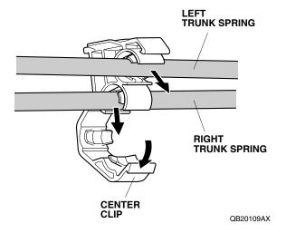
28. Put on heavy gloves to protect your hands. With an assistant holding the trunk lid open, remove both trunk springs with the trunk spring tool. Pull the trunk spring tool slowly and carefully toward you. First remove the right trunk spring, then remove the left trunk spring.
