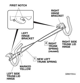
30. Reinstall the center clip to the trunk springs.
