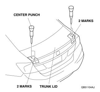
8. While wearing eye protection, drill four 8.5 mm holes at the center-punched marks with an 8.5 mm hole cutter. Drill perpendicular to the trunk lid.
