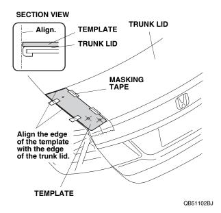
4. Using a felt-tip pen, mark the trunk lid through the template at the two locations shown on the template.
