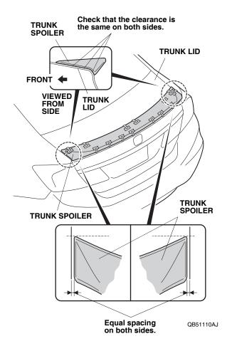
15. While applying light pressure against the trunk spoiler, carefully remove the bottom adhesive backings shown.
