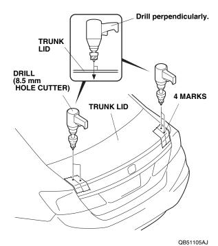
9. Remove the tape installed in step 2. Remove all burrs and metal shavings with a file, and apply touch-up paint to the edges of the holes.
