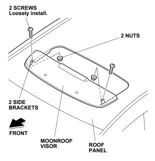
14. Position the moonroof visor with equal spacing on each sides. Check that the rubber molding is not twisted or rolled under the visor.
