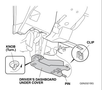
13. Remove the driver's dashboard lower cover and unplug the vehicle connectors.
