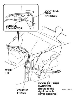
54. Route the door sill trim harness, and secure it to the vehicle frame with two wire ties.
