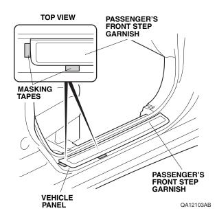
8. Pull away the door opening seal, and remove and discard the passenger's front step garnish.
