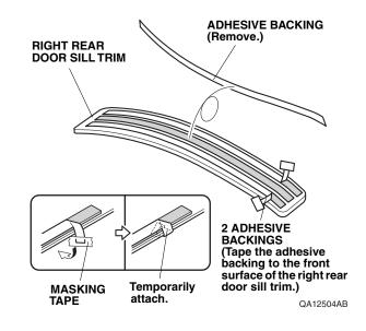
33. Using one alcohol swab, thoroughly clean the right rear step garnish where the right rear door sill trim will attach.
