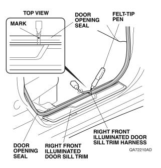
21. Pull away the door opening seal, and remove the right front illuminated door sill trim.
