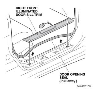
22. Using an utility knife, cut the door opening seal at the mark made in step 20.
