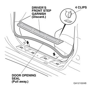
17. Pull away the door opening seal, and remove the driver's kick panel.
