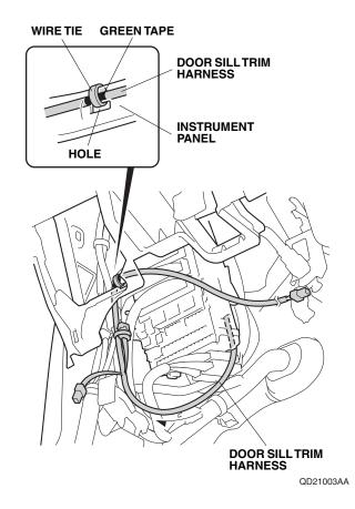
44. Secure the door sill trim harness to the vehicle harness with three wire ties.
