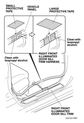
29. Using isopropyl alcohol on a shop towel, thoroughly clean the small protective tape where the large protective tape will attach. Secure the right front illuminated door sill trim harness to the vehicle panel with the large protective tape as shown.
