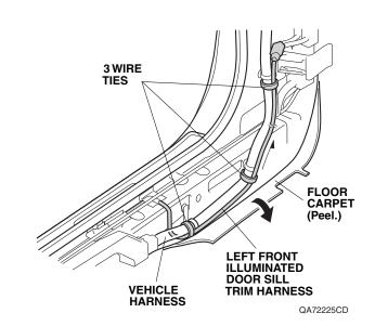
48. Route the left front illuminated door sill trim harness, and secure it to the vehicle harness with three wire ties.
