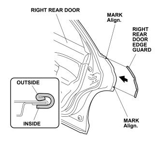
14. Starting at the feature line, tap the right rear door edge guard into position with a series of light taps using a rubber mallet, then work up and down. Make sure the position of the right rear door edge guard is correct. Once in place, do not remove, reposition, or reinstall the right rear door edge guard.
