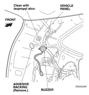
56. Remove the adhesive backing from the buzzer and attach the buzzer to the vehicle panel in the location shown.
