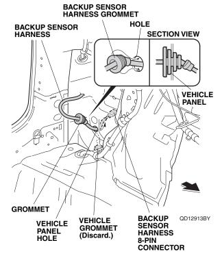
30. Route the backup sensor harness 8-pin connector through the hole, and seat the backup sensor harness grommet into the vehicle panel hole. NOTE: Do not pull on the backup sensor harness when installing the grommet. 31. Adjust the volume control knob on the control unit as shown.
