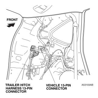
46. Plug the backup sensor harness 13-pin connector into the vehicle 13-pin connector.
