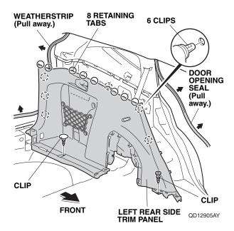
17. Release the wire and remove the lever, then remove the left rear side trim panel.
