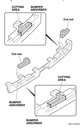
89. Reinstall the bumper absorber to the rear bumper beam.
