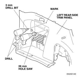
64. Install the switch into the 26 mm hole in the left rear side trim panel.
