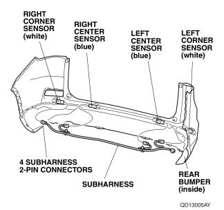
81. Secure the two subharness clips into two center sensor clips.
