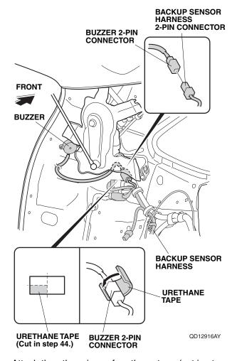
53. Attach the other piece of urethane tape (cut in step44) around the buzzer 2-pin connector.
