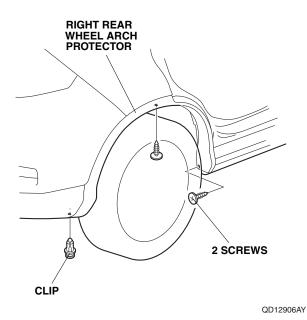
22. Remove the one clip and the two screws from the right rear wheel arch protector. If equipped, remove the splash guards.
