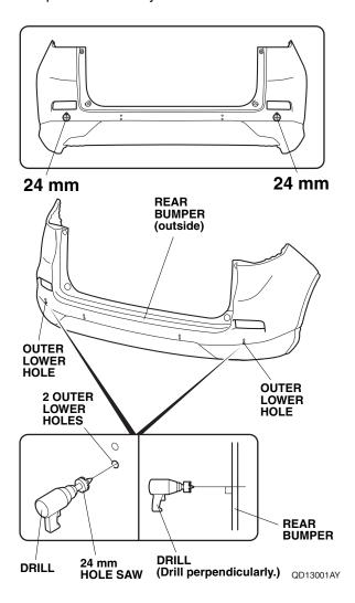
75. While wearing eye protection and drilling from painted side of the rear bumper, enlarge the two lower 3 mm inner holes to 26 mm using a 26 mm hole saw.
