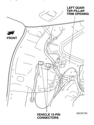
43. Slide the clip from the backup sensor harness 13-pin connector onto the vehicle connector clip.
