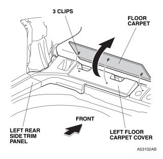
11. Remove the left floor carpet cover (three clips and two retaining tabs).
