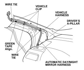
25. Align the green tape on the automatic day/night mirror harness with the upper vehicle clip, and secure the automatic day/night mirror harness to the vehicle harness with three wire ties.
