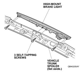
9. Install the high-mount brake light to the new trunk spoiler with the three self-tapping screws removed in step 8.
