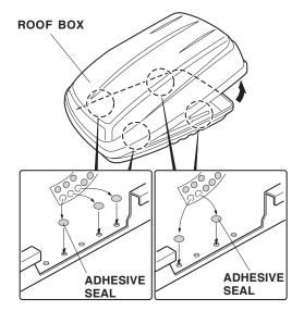
Using isopropyl alcohol on a shop towel, clean the four brackets B where the small pads will attach. Remove the adhesive backing from the small pads, and attach them to brackets B.
