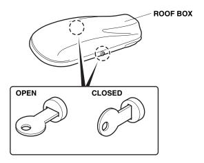
**Locking:** Press down on the lid. There should be an audible click. Be sure the lid is latched by attempting to lift the lid. Turn the key clockwise to lock the roof box. Remove the key while not in use. Make sure the straps do not dangle from the roof.
