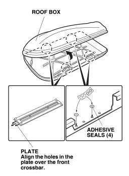
3. Attach an adhesive seal over the unused rear mounting holes along the bottom of the roof box. The seals will help prevent water from entering the roof box. Remove the roof box from the vehicle.
