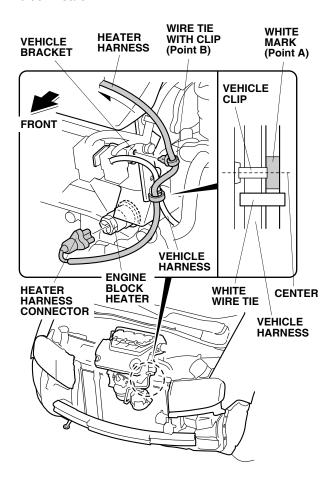
12. Route the heater harness up, and secure it to the vehicle harness with one white wire tie (Point A). Secure the heater harness to the vehicle bracket with one wire tie with clip (Point B).
