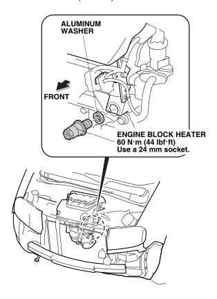
11. Plug the heater harness connector into the engine block heater.
