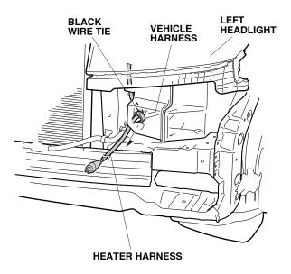
18. Route the heater harness along the vehicle harness, and secure it to the vehicle harness with one black wire tie (Point F).
