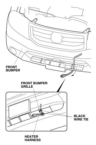
21. Route the heater harness through the front bumper, and secure it to the front bumper grille with two black wire ties.
