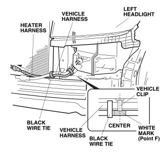
19. Secure the heater harness to the vehicle harness with one additional black wire tie.
