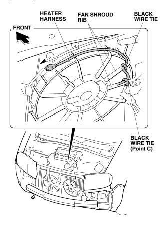
14. Secure the heater harness to the next fan shroud rib with one additional black wire tie.
