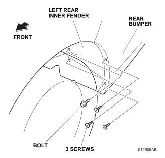
Secure the left rear splash guard to the left rear inner fender and rear bumper with one 5 x 25 mm selftapping screw, one bolt removed step in 1 and two screws removed step in 1. While holding the splash guard firmly against the fenderwell, tighten the selftapping screw, screws and bolt in the order
