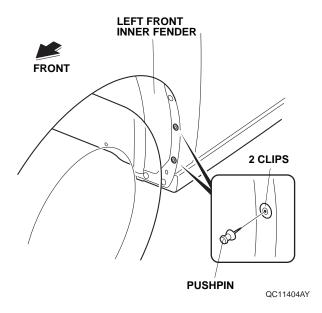
8. Secure the left front splash guard to the left front inner fender with one 5 x 25 mm self-tapping screw and three screws removed step in 1 and step in 6. While holding the splash guard firmly against the fenderwell, tighten the self-tapping screw and screws in the order 1 → 2 → 3 → 4.
