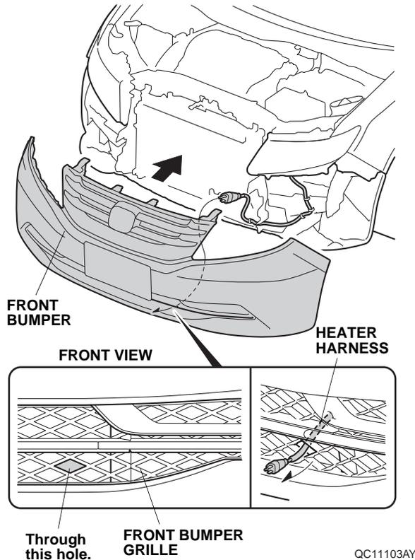
29. Attach the protective cap to the front bumper grille.
