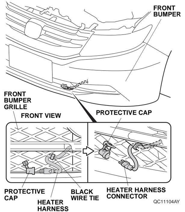
30. Secure the heater harness to the front bumper grille with one black wire tie, and plug the heater harness connector into the protective cap.
