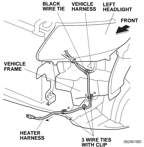
26. Secure the heater harness to the vehicle frame with three wire ties with clip.
