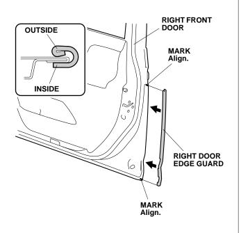
8. Starting at the feature line, tap the right door edge guard into position with a series of light taps using a rubber mallet, then work up and down. Make sure the position of the right door edge guard is correct. Once in place, do not remove, reposition, or reinstall the right door edge guard.
