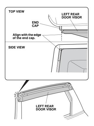
17. While holding the door visor up firmly, remove the adhesive backing in the order shown. Use your finger to push up each bracket so there is no gap between the brackets and the door sash.
