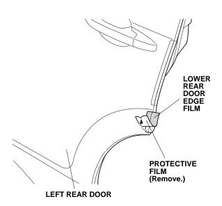
23. Starting from the middle of the lower door edge film and working outward, fold the door film around the edge using your fingers. Move your fingers in one direction. Attach the film over the seam sealant. Do not trim or damage the seam sealant.
