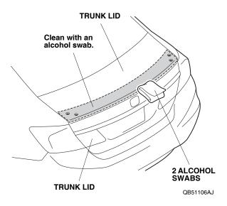
11. Get the trunk spoiler and the four clips. Install the four clips to the trunk spoiler.
