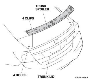
14. Visually check that the clearance between the trunk spoiler and the trunk lid is the same on both sides. If necessary, adjust the position of the trunk spoiler until there is equal spacing on each side.
