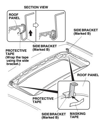
9. Place the two front brackets (marked A) into position over the protective tape and around the lip of the roof opening, and tape them into position with a piece of masking tape. Be sure to align the lower end of the front brackets with the indentation in the lip.
