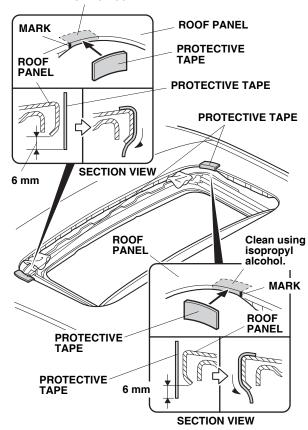
Remove the adhesive backings from two pieces of protective tape, and attach them to the roof panel at the two marks you made. Allow 6 mm of each protective tape to hang below the bottom lip of the roof panel. Remove the marks.  Locate the third indentations along the front edge of the moonroof opening. Using isopropyl alcohol on a shop towel, clean the roof area and the inside edge of the moonroof opening where the protective tapes will attach.
