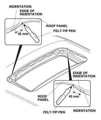
4. Using isopropyl alcohol on a shop towel, clean the roof panel at each of the two marks you made, but don't wipe off the marks.
