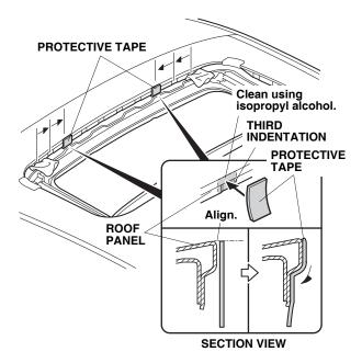
7. Remove the adhesive backing from one of the protective tapes. Starting at the top edge of the moonroof opening, wrap one protective tape around the lip of the moonroof opening to cover one of the located indentations.
