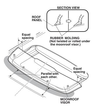
14. While holding the side brackets against the roof panel, tighten the two screws and nuts on the side bracket. While holding the front brackets against the roof panel, tighten the two screws and nuts on the front brackets. Using a torque screwdriver, torque all of screws to 2.0 N·m (1.5 lbf·ft).
