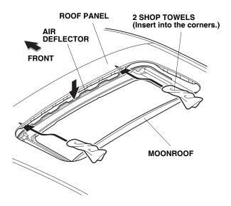
Locate the edge of the indentation on the right side and left side of the moonroof opening. Measure 40 mm (1.6 in.) to the front of the vehicle, and make one mark on each side of the roof panel.
