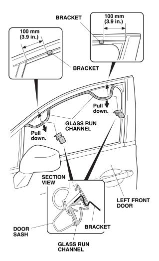
2. Install two brackets between the door sash and the glass run channel at the measurements shown. Seat the glass run channel properly around the brackets.
