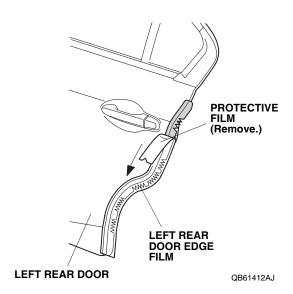
14. Starting from the center and working outward, use your fingers to fold the left rear door edge film around the edge of the left rear door as shown. Move your fingers in one direction only. Attach the left rear door edge film over the seam sealant. Do not trim or damage the seam sealant.
