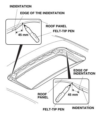
4. Using isopropyl alcohol on a shop towel, clean the roof panel at each of the two marks you made, but don't wipe off the marks.
