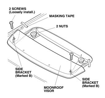
13. Position the moonroof visor with equal spacing on all sides. Check that the rubber molding is not twisted or rolled under the moonroof visor.
