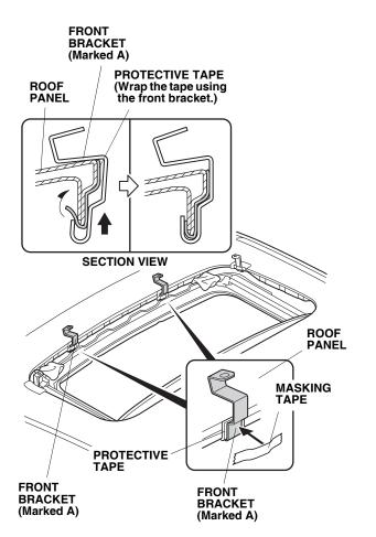
11. Set the moonroof visor on the vehicle roof in front of the moonroof opening, and adjust its position so the holes in the moonroof visor are aligned with the bracket holes. Loosely install the moonroof visor onto the front bracket (marked A) with two screws and two nuts. Remove the masking tape.
