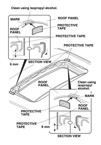
5. Remove the adhesive backings from two pieces of protective tape, and attach them to the roof panel at the two marks you made. Allow 6 mm of each protective tape to hang below the bottom lip of the roof panel. Remove the marks.
