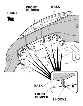
5. On each side, attach one hook to the hole in the front bumper.
