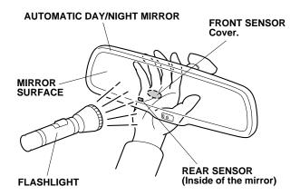
4. With the parking brake properly set, step on the brake pedal, and move the select lever to the "R" position. Repeat step 3, and check to make sure the mirror surface does not become dim. If the automatic day/night mirror does not function properly, check the fuse and all the connectors.
