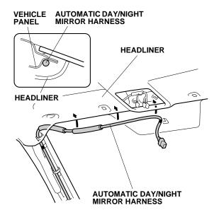
28. Align the green tape on the automatic day/night mirror harness with the edge of the headliner. Be careful not to crease the headliner.
