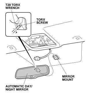
31. Plug the automatic day/night mirror harness 7-pin connector into the automatic day/night mirror.
