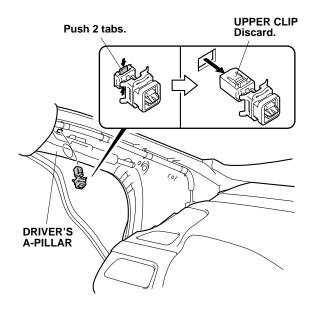
12. Remove the driver's dashboard panel (six clips and unplug the vehicle connector).
