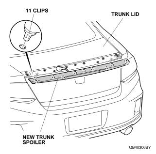
16. Open the trunk lid. Secure the new trunk spoiler to the trunk lid with the two bolts removed in step 3. Torque the bolts to 5 N·m (3.7 lbf·ft).
