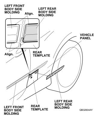
14. Check that the edges of the front and rear moldings are aligned. Readjust the moldings if necessary.
