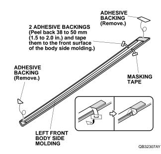
Align the left front body side molding with the front template, and attach it to the left door as shown.
