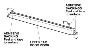
13. Using isopropyl alcohol on a shop towel, clean the door sash where the left rear door visor will attach.
