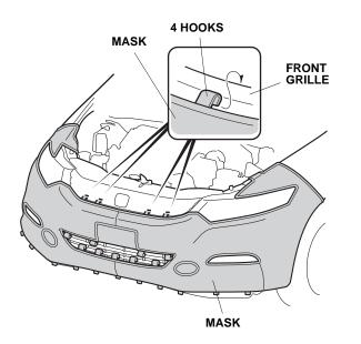
14. Secure the seven hooks to the front lower grille.
