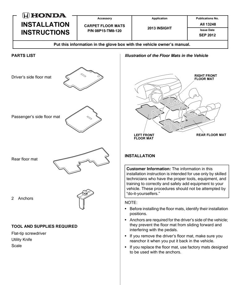
1. Install the driver's side floor mat over the anchors as shown.
