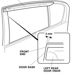
19. While holding the door visor firmly in position, remove the adhesive backing. Use your finger to push up each bracket so there is no gap between the brackets and the door sash.
