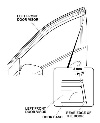
9. While holding the door visor firmly in position, remove the adhesive backings. Use your finger to push up each bracket so there is no gap between the bracket and the door sash.
