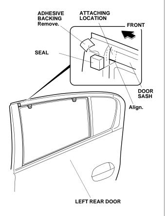
16. Peel back approximately 1-1½ inches of adhesive backing from each adhesive strip, and tape the ends to the front surface of the left rear door visor.
