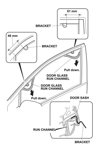
3. Install two brackets between the door sash and the run channel at the measurements shown. Then seat the door glass run channel properly around the brackets.
