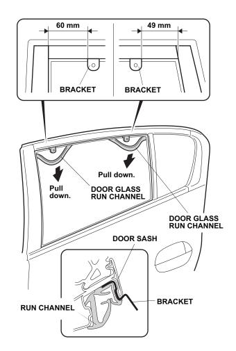
13. Install two brackets between the door sash and the run channel at the measurements shown. Then seat the run channel properly around the brackets.
