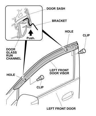
8. Adjust the left front door visor to the position shown.
