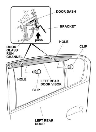
18. Adjust the left rear door visor to the position shown.
