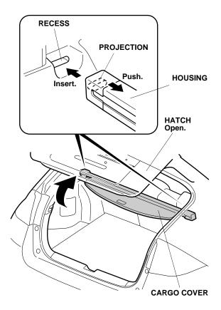
2. Insert the left end of the cargo cover into the recess in the left rear side trim panel. Push the end further into the recess, hold it in that position, then insert the right end into the recess in the right side trim panel.
