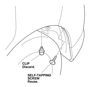
11. With the vehicle on a lift, temporarily install the left rear splash guard using one clip, the self-tapping screw from step 10, and a strip of masking tape. Make sure there is no gap between the left rear splash guard and the vehicle.
