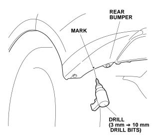
While wearing eye protection, drill a 10 mm hole through the left rear splash guard. First drill with a 3 mm drill bit, then finish with a 10 mm drill bit. Remove all burrs.
