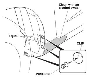
2. Using a pushpin, make small holes through the centers of the three clips on the left front inner fender.
