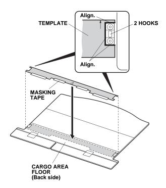
11. Using a utility knife, cut the cargo area floor along the edge of the template.
