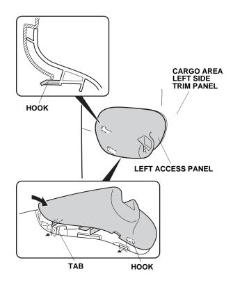
• Push the left access panel in the direction shown to lock three tabs.
