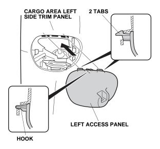
• Insert one tab, and install two hooks.
