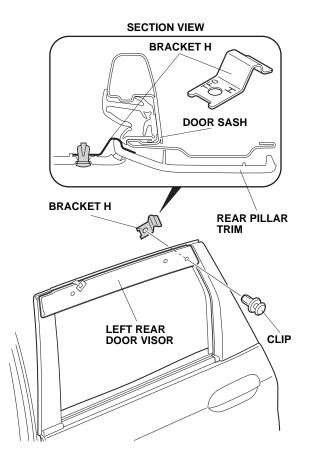
21. While pressing the left rear door visor in the direction of the arrow make sure there is no gap between the brackets and the door sash. Remove the adhesive backing
