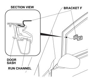
28. Using isopropyl alcohol, clean the door sash where the left front door visor will attach.
