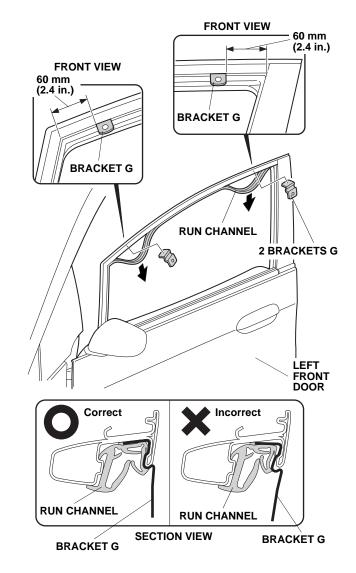
25. Install two brackets G to the door sash at the measurements shown.
