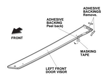
31. Secure the left front door visor to two brackets G with two clips.
