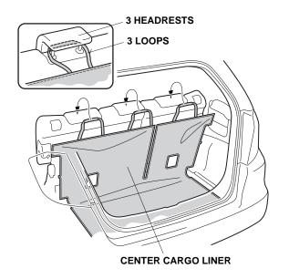
Pull the knobs and fold down the left and right seatbacks. Position the center cargo liner on the left and right seat-backs. Secure the center cargo liner to the left and right seat-backs with 10 hook-and-loop fasteners.
