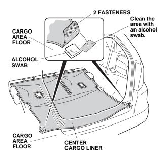
7. Attach two fastener pads to the center cargo liner fasteners as shown.
