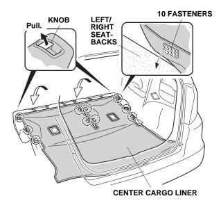
3. Position the center cargo liner on the cargo area floor. Secure the center cargo liner to the cargo area floor with six hook-and-loop fasteners.
