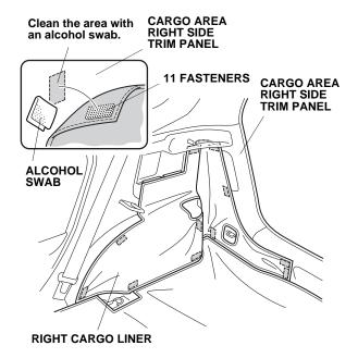
14. Attach 11 fastener pads to the fasteners on the right cargo liner as shown.
