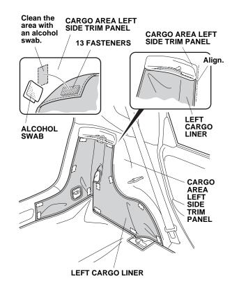
10. Attach 13 fastener pads to the fasteners on the left cargo liner as shown.
