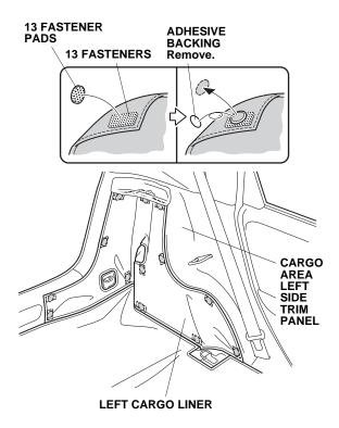
11. Remove the adhesive backings from the 13 fastener pads, position the left cargo liner, and attach the 13 fastener pads to the cargo area left side trim panel.
