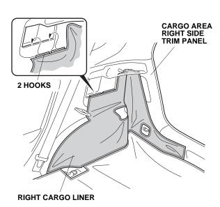
13. Position the right cargo liner on the cargo area right side trim panel. Fold back the edge of the right cargo liner. Using an alcohol swab, clean the areas where the 11 fastener pads will attach.
