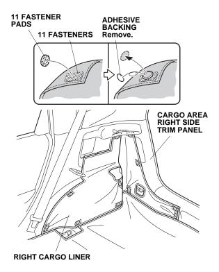
15. Remove the adhesive backings from the 11 fastener pads, position the right cargo liner, and attach the 11 fastener pads to the cargo area right side trim panel.
