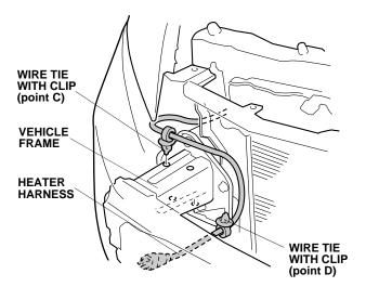
Bundle the excess of the heater harness. Using three black wire ties, secure the harness to the vehicle harness.
