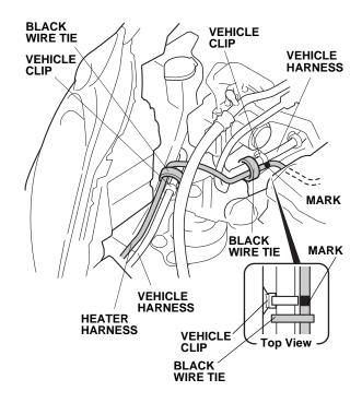
15. Route the heater harness as shown and secure the two wire ties with clips (points C and D) to the vehicle frame.
