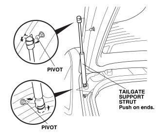
• Repeat this procedure to install the tailgate support strut on the other side of the vehicle.
