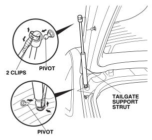
Set the ends of the new tailgate support strut on the pivots, then push on the ends to attach the strut to the pivots.
