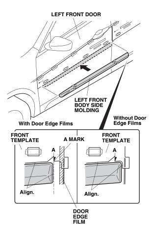
10. Press the left front body side molding firmly with the palm of your hand and remove the adhesive backing 50 to 100 mm (2 to 4 in.) at a time.
