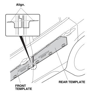
7. Using two alcohol wipes, clean the door surfaces below the templates where the body side moldings will attach. Allow the alcohol to dry.
