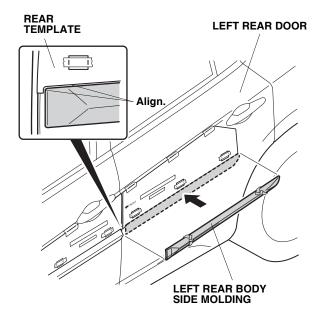
14. Press the left rear body side molding firmly with the palm of your hand and remove the adhesive backing 50 to 100 mm (2 to 4 in.) at a time.
