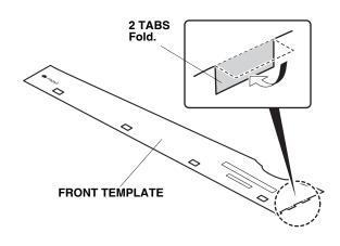
2. Insert the two tabs on the front template around the rear edge of the left front door.
